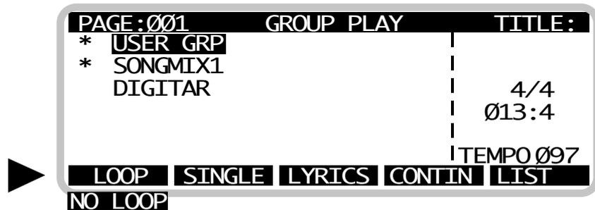
In order to enable one of the Soft Key commands, just press the SOFT KEY relevant to the desired command.
