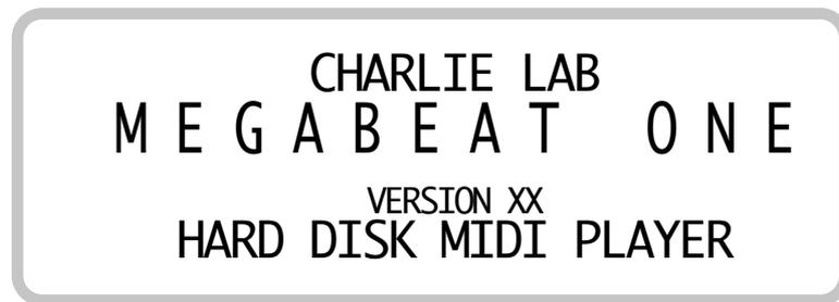
Don't worry if after turning on, no message appears on the display. The instrument is checking the hard disk and the Ram and this operation can last up to a minute.
